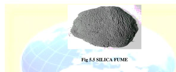
There are two reactions in the silica fume, Pozzolanic reactions are, Silica fume reacts with the calcium hydroxide, which is liberated during process of Hydration, about 22-24 percent and produces calcium-silicate-hydrate (C-S-H). The following are the chemical reactions that are taking place.
